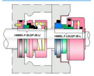
HM05KL-F seal instead of original Flygt seal used for Flygt pump no:2084/ 2135/2151-01 1/2151-050
